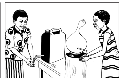
To start water flow, remove container before you pour water in the lid or plug. To stop water flow, put tight the container lid.
